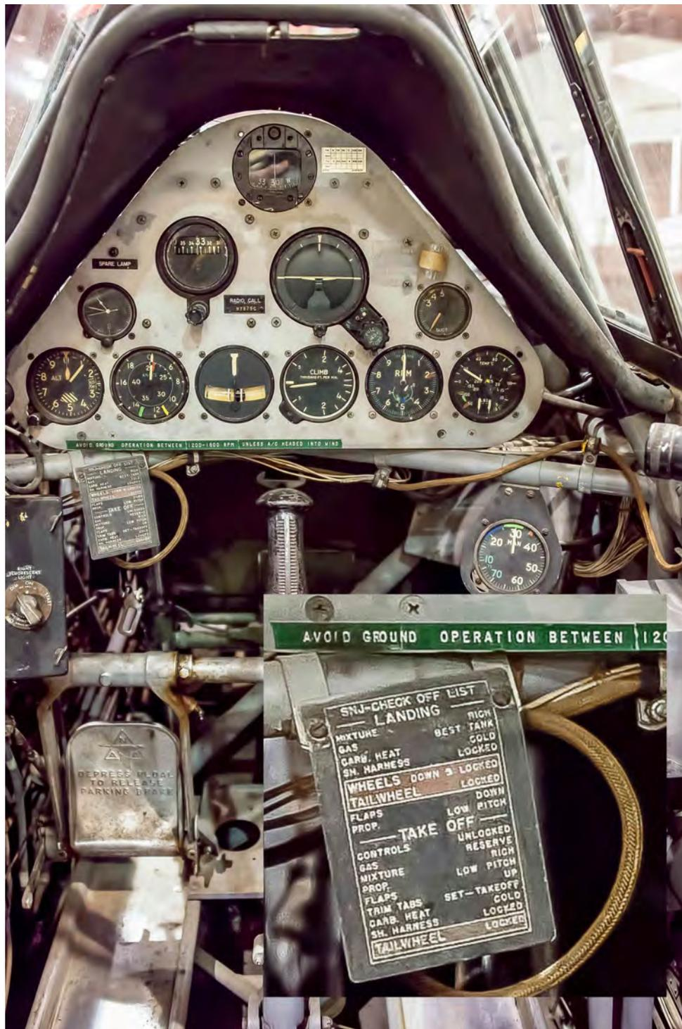
Figure 6 Cockpit of SNJ trainer. Checklist shown in inset.
